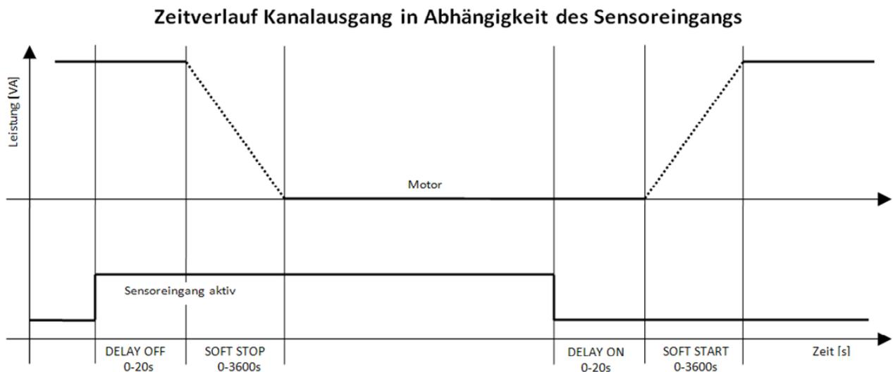
Figure 1: Time curve for load output, sensor input
